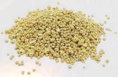
Brass in granulated form (67% copper 33% zinc)
