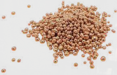
Bronze in granulated form (90% copper 10% tin)
